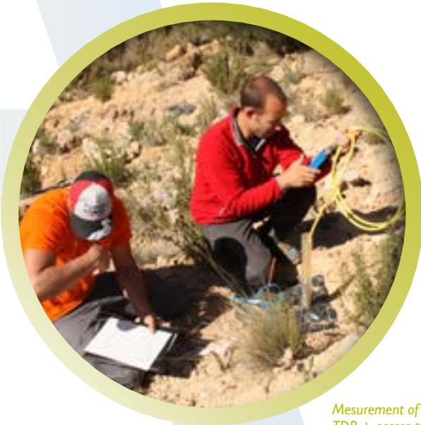
*Measurement of soil moisture with TDR + access tube*
