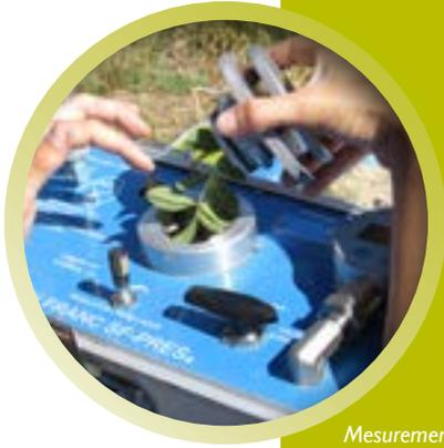
*Measurement of leaf water potential with pressure chamber*
