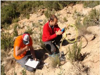
Monitoring Sustaffor field trials: measurement of tree diameter with digital calliper and soil moisture with TDR probe
