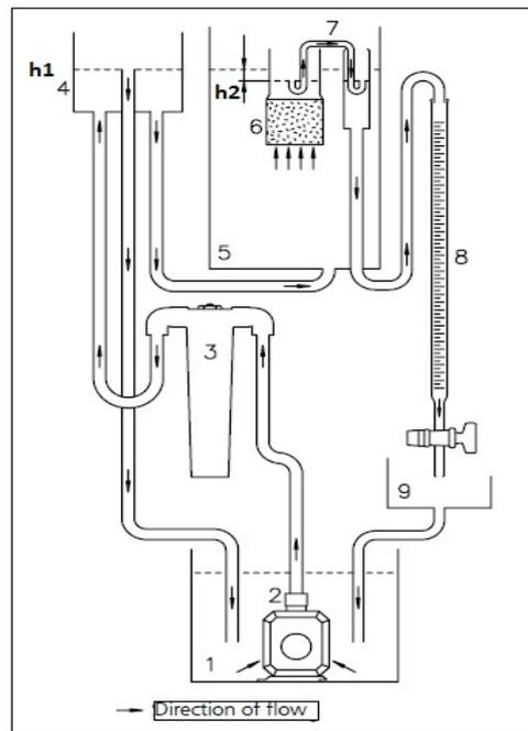
This device is specifically designed to measure the saturated hydraulic conductivity  $K_s$ . The saturated samples (1) are placed under the influence of a constant water head (2). An upward water flow (3) is forced through the samples based upon the law of communicating vessels. The  $K_s$  (m/s) can be calculated using the formula:
